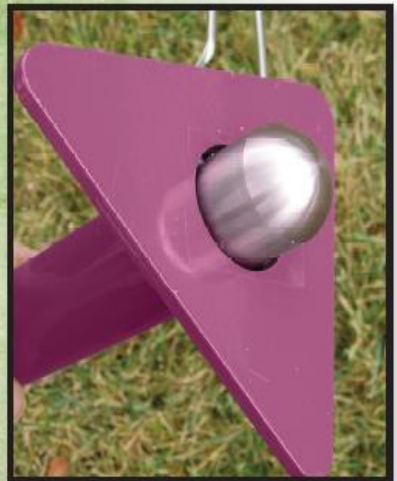
Golf Ball Shaped Hammer for Better Impact Simulation
