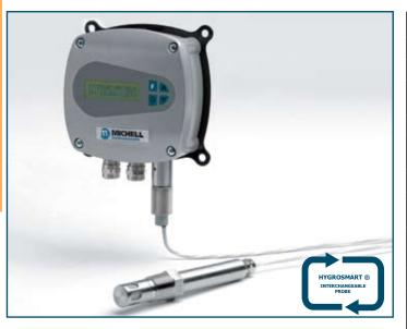
The WR295 relative humidity transmitter includes the interchangeable HYGROSMART module. This interchangeable module allows you to recalibrate the transmitter simply by replacing the sensor head. As a result, maintenance costs are greatly reduced and down-time is minimized.
