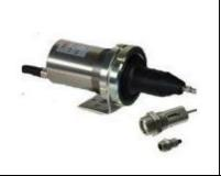
CellaTemp PA 21 is a digital pyrometer featuring fibre optics to measure temperatures ranging from 350 to 2000 °C. The sensor head is housed separately from the electronics assembly. Both the sensor head and the fibre optic cable are unsusceptible to electromagnetic radiation. The optical sensor head can withstand ambient temperatures up to 250 °C without cooling. CellaTemp PA 31 is ideal for cramped, hard-to-access locations.
