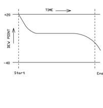
dewpoint between the inlet value and the outlet value is used as an indicator of pipeline dryness. It is common for a differential of 5°C dewpoint to be used as the signal to end the drying process.
