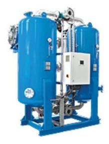
Regenerative desiccant column dryers can offer a very efficient method of air drying. These dryers are normally configured in twin columns, allowing one column of desiccant to be regenerated while the other is performing the air drying process. There are two common types - pressure swing and heat regenerative. A pressure swing dryer uses a sudden drop in pressure of the column under
