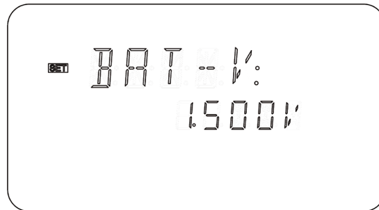
Figure 5-3 Set up cut-off voltage
