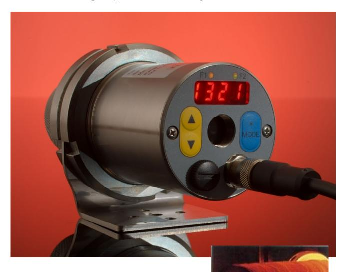
High-precison temperature measurement of reflective metals and silicon wafers
