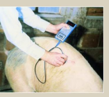
The Renco *Lean-Meater* makes backfat measurements by using high frequency sound waves (called "ultrasound"). The animals are neither hurt or irritated. Ultrasound is safe; no piercing the skin, no danger of infection.
